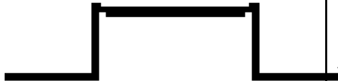
Frequency Spectrum of a Chirp Signal
