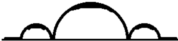
Frequency Spectrum of a Direct Sequence Signal
